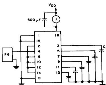
Fig. 9—Dynamic power dissipation test circuit.
