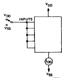
Fig. 10—Quiescent-device-current test circuit.
