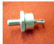
1N4510 Standard Rectifier (trr More Than 500ns)
