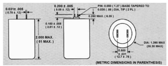
UP37 uses straight feed through mounting tabs
