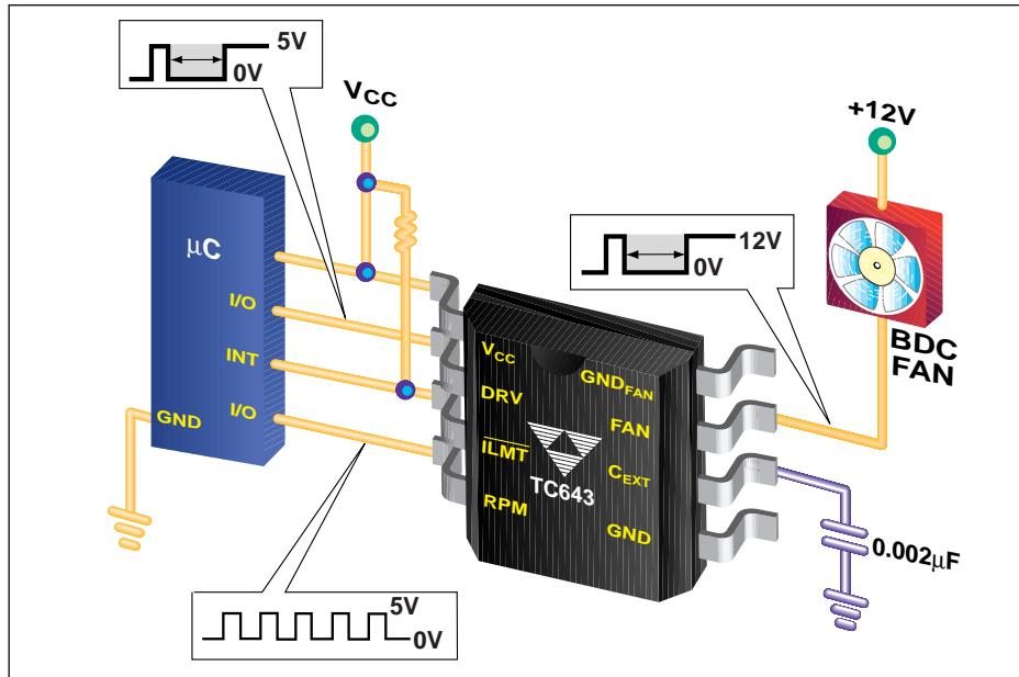
The TC643 is a switchmode brushless DC fan/motor speed driver with diagnostic circuits. External components are kept to a minimum by integrating the power transistor on chip. Any logic-level signal can be used to drive the on-chip Power Driver. The output is current limited and a logic-level indication, ILMT, is provided to indicate an over-current condition.
