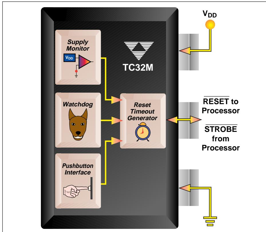
The TC32M is the industry's first processor supervisor to incorporate a power supply monitor, reset generator (with external override) and watchdog timer in a 3-pin package. Available in a TO-92 package and SOT-223 package, the TC32M offers the same functionality as the industry standard, TC1232, but in a smaller, lower cost configuration.
