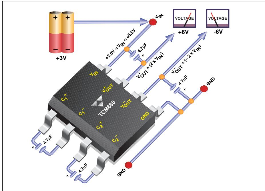
The TelCom TCM680 is a dual-capacitive charge pump converter that develops  $\pm 10V$  from a single  $+5V$  logic power supply or  $\pm 6V$  from a  $+3V$  lithium cell. The TCM680 requires only four inexpensive electrolytic capacitors and no inductors.
