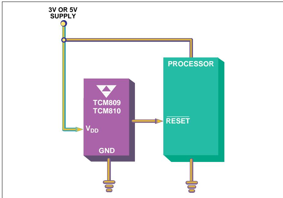
The TCM809/810 are cost-effective processor supervisor circuits that monitor the supply voltage in digital systems and provide a processor reset signal when necessary. No external components are required. The TCM809 has an active low reset output, while the TCM810 has an active high reset output.
