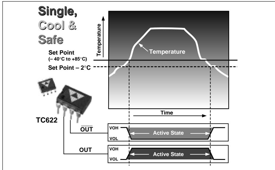
The TC622 integrates a temperature sensor, voltage reference, and all required circuitry to form a stand-alone, single trip-point temperature sensor.
