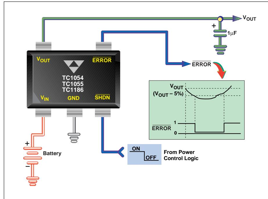
The TC1054/1055/1186 are CMOS upgrades to bipolar low dropout regulators such as the LP2980. CMOS construction guarantees no ground current as in bipolar regulators, resulting in significantly lower supply current over the entire load range. Maximum output currents of 50mA (TC1054), 100mA (TC1055), and 150mA (TC1186) are available. Typical dropout voltage is 85mV (TC1054), 180mV (TC1055), and 270mV (TC1186) at full load. An output capacitor of only 1μF is required for stability.
