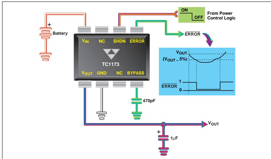
The TC1173 is a precision output (typically  $\pm 0.5\%$ ) CMOS low dropout regulator. Designed specifically for battery-operated systems, the TC1173's CMOS construction eliminates wasted ground current, significantly extending battery life. Total supply current is typically  $50\mu\text{A}$  at full load (*20 to 60 times lower than in bipolar regulators!*).
