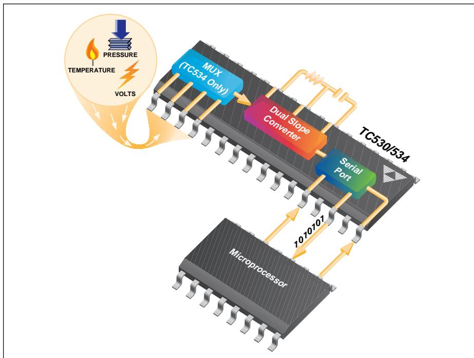
The TC530/534 are low cost 5V serial data acquisition systems targeted at precision measurement applications. The TC530 and TC534 utilize dual slope integration conversion technology and deliver 17-bit accuracy with greater than 60db of 50/60Hz noise rejection. The user can readily adapt the TC530/534 to the measurement task at hand by trading off decreased resolution for faster conversion time.
