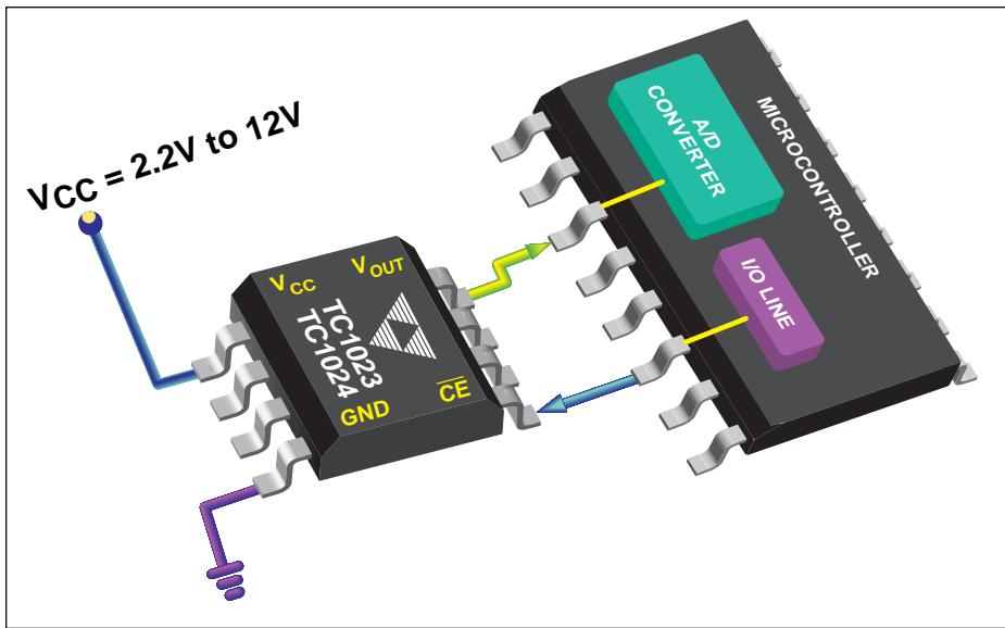
The TC1023/1024 temperature sensors furnish a linearized output voltage directly proportional to measured temperature. The TC1023 has a temperature measurement range of – 20°C to +100°C. Its output voltage is directly calibrated in degrees Centigrade (i.e.,  $V_{OUT} = 10mV/^{\circ}C \times \text{Temperature } ^{\circ}C$ ). An external pull-down resistor to a negative voltage source is required for temperature measurement below 0°C.
