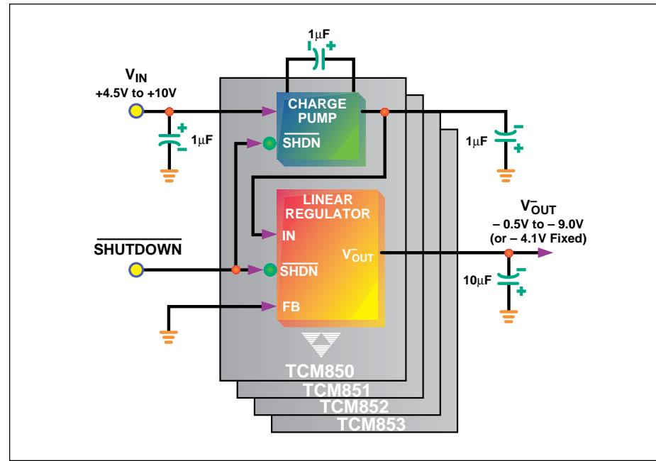
The TCM850/851/852/853 combine an inverting charge pump and a linear post-regulator in a single 8-pin SOIC package. The regulated, low noise output makes these devices ideal in GaAs FET bias applications. They work particularly well in GSM phones, where the devices' output may also be used as the reference for a digital-to-analog converter (DAC).
