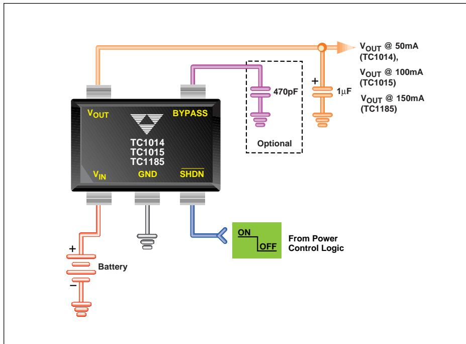
The TC1014/1015/1185 are CMOS upgrades to bipolar low dropout regulators, such as the LP2980. CMOS construction guarantees no ground current, as in bipolar regulators, resulting in significantly lower supply current over the entire load range. A reference bypass input also is provided for excellent low noise operation.
