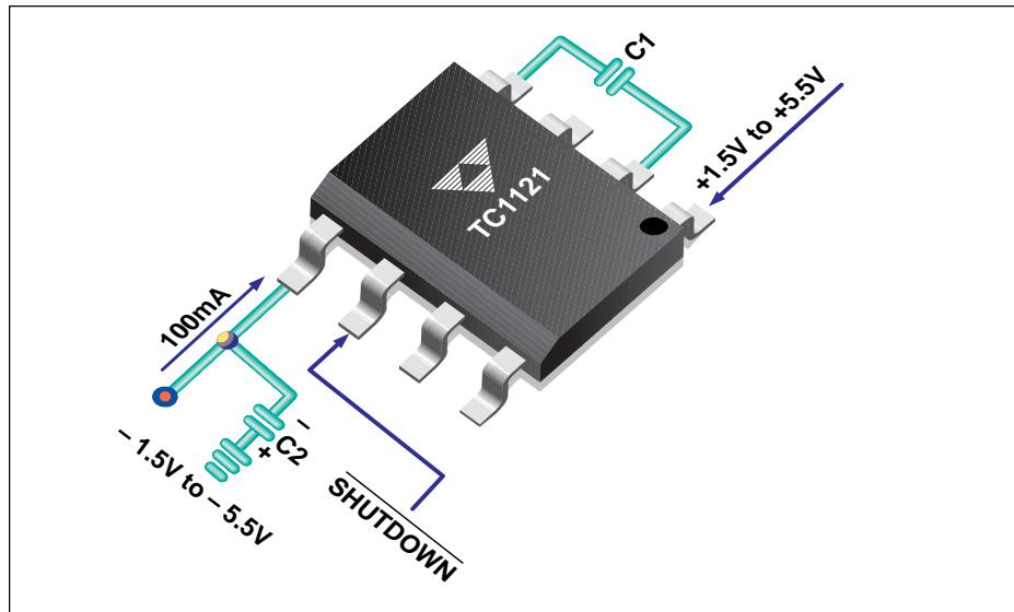
The TC1121 charge pump converter is a higher output current upgrade to the MAX860 and similar charge pump devices. It is capable of supporting a 100mA output load. Typical applications include voltage inverters and doublers from an input voltage range of 1.5V to 5.5V. As with all charge pump converters, the TC1121 uses no inductors which saves cost, size and EMI.
